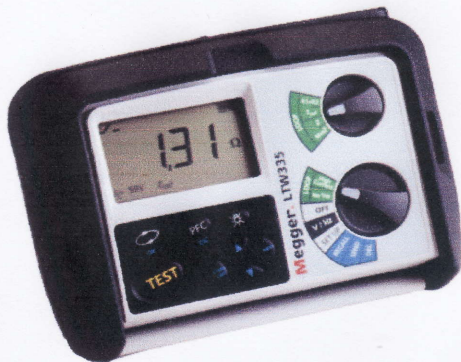
7. Megger meter ( for insulation Test )
